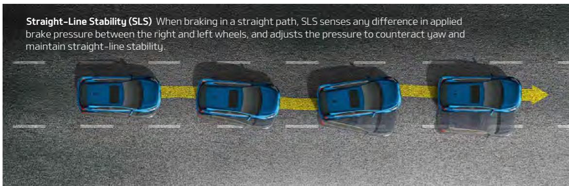
**Straight-Line Stability (SLS)** When braking in a straight path, SLS senses any difference in applied brake pressure between the right and left wheels, and adjusts the pressure to counteract yaw and maintain straight-line stability.
